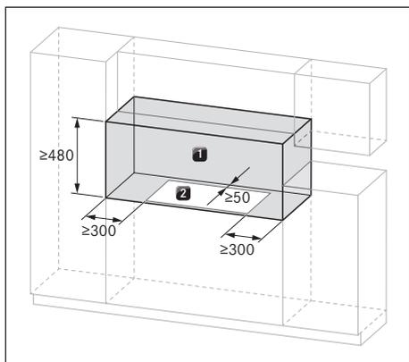
Fig. 6.5 Required clearance
