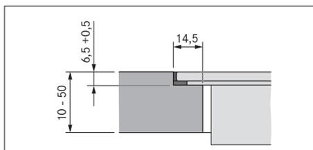
Fig. 6.7 Dimensions of groove for flush installation
