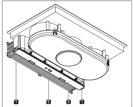
Fig. 8.5 Releasing the activated charcoal filter housing lid
