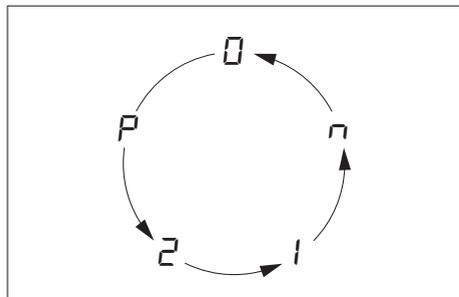
Fig. 7.2 Fan level sequence
