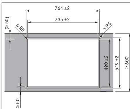
Fig. 6.6 Dimensions of cut-out for flush installation
