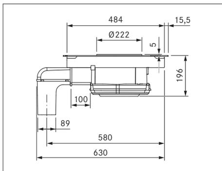
**Fig. 3.4** Device dimensions with cable extension (BHA + BLAVH1)
