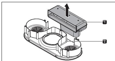
**Fig. 6.33** Removing the exhaust air arc
