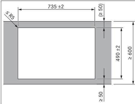
Fig. 6.8 Dimensions of cut-out for surface installation
