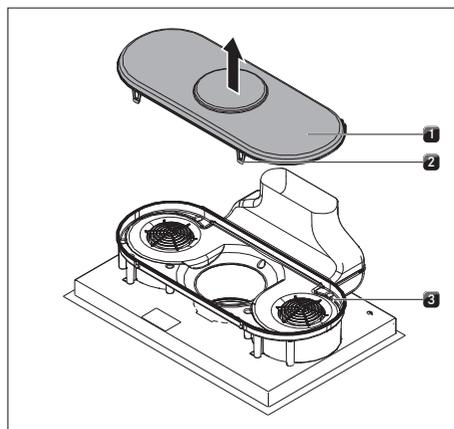
Fig. 6.29 Removing the housing base
