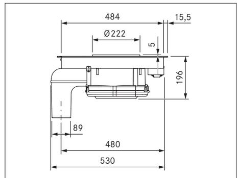
Fig. 3.3 BHA Device dimensions side view
