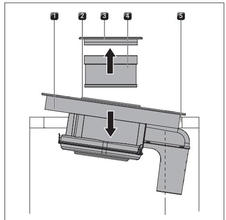
**Fig. 6.38** Inserting the cooktop
