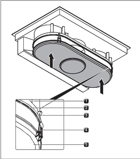
Fig. 8.4 Closing the air guiding housing
