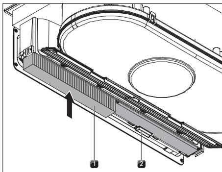
**Fig. 8.9** Inserting the activated charcoal filter
