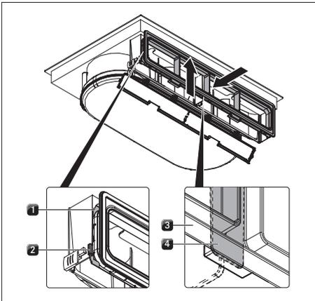
Fig. 6.17 Mounting the frame of the flexible duct
