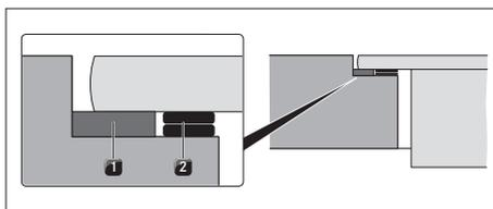
Fig. 6.21 Height adjustment plates
