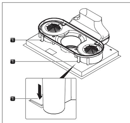
Fig. 6.30 Releasing the position lock
