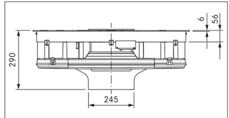
Fig. 3.2 BHA Device dimensions front view
