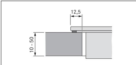
Fig. 6.9 Dimension of support for surface installation
