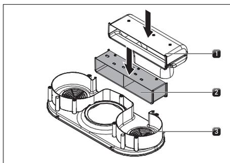
**Fig. 6.34** Inserting the extension for exhaust air duct
