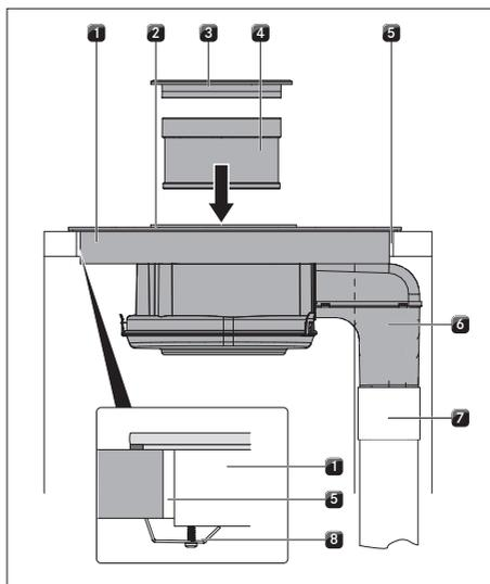
Fig. 6.40 Connecting the exhaust air duct + secure
