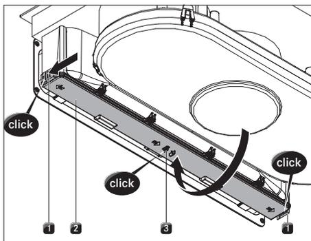
**Fig. 8.10** Closing the activated charcoal filter housing cover
