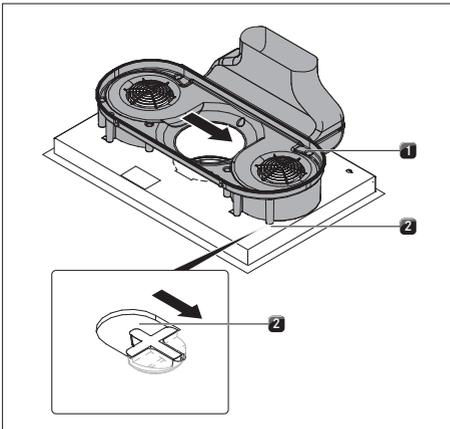
**Fig. 6.36** Engaging the airflow assembly
