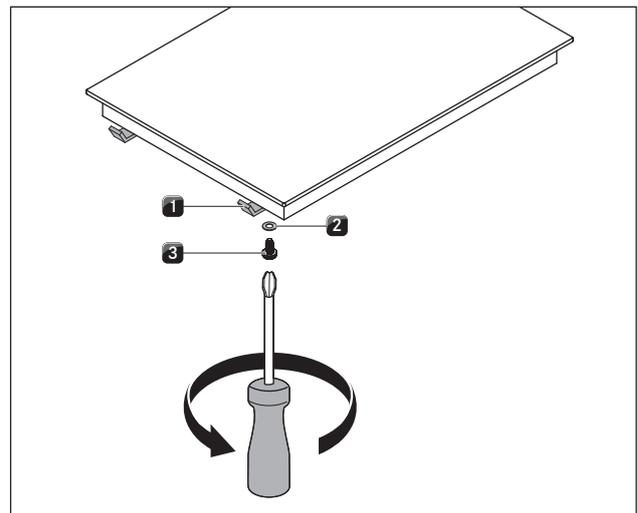
Fig. 5.16 Mounting brackets
