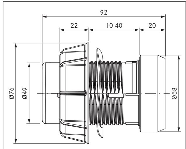
Fig. 3.7 Device dimensions control knob
