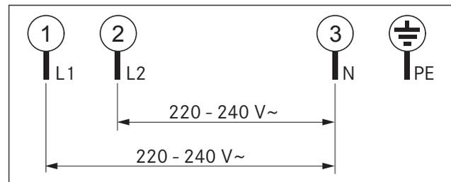
Fig. 5.23 Connection diagram 2-phase
