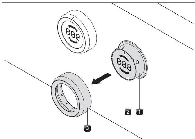
Fig. 7.5 Pull out the knob ring
