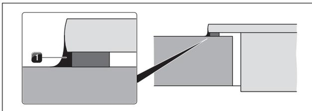
Fig. 5.26 Silicone sealant for surface mounting
