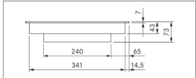
Fig. 3.5 PKC3B Device dimensions front view
