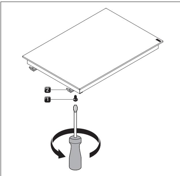
Fig. 5.16 Mounting brackets
