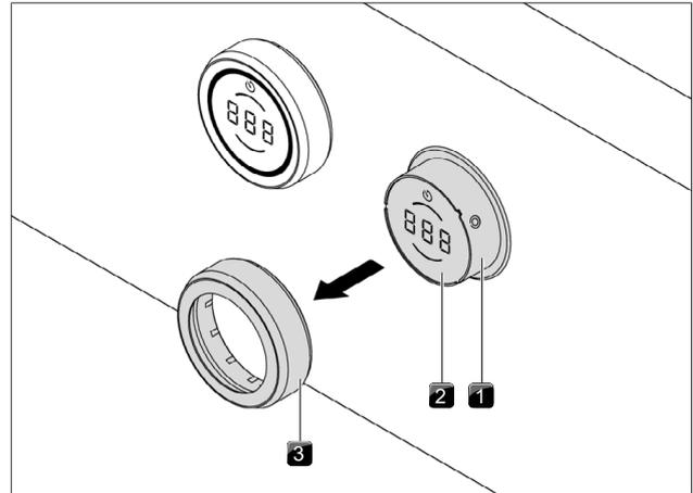
Fig. 7.8 Pull out the knob ring
