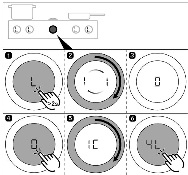
Fig. 5.19 Permanently deactivating the child lock
