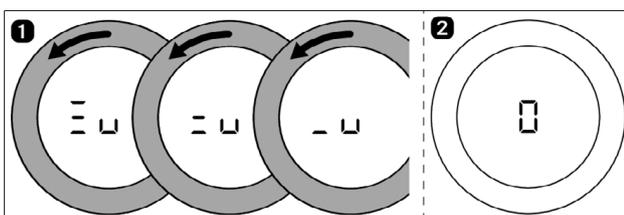
Fig. 5.35 Deactivating the heat retention function
