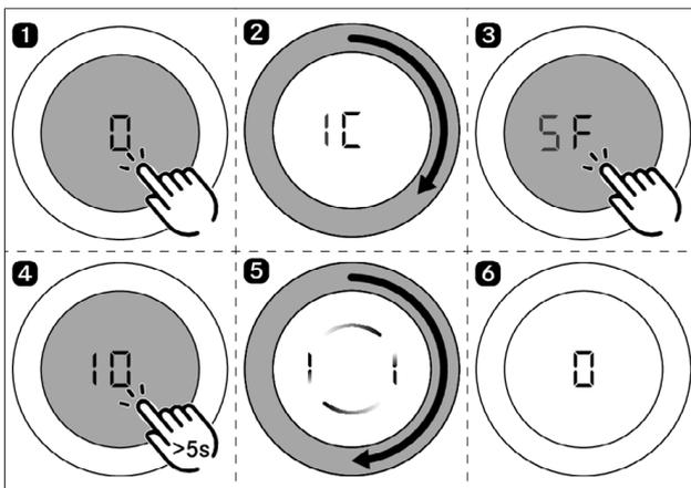
Fig. 5.21 Resetting the filter service life early
