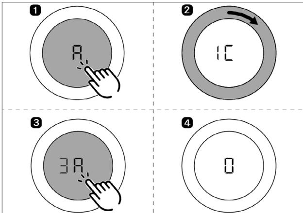
Fig. 5.16 Deactivating the automatic extractor function
