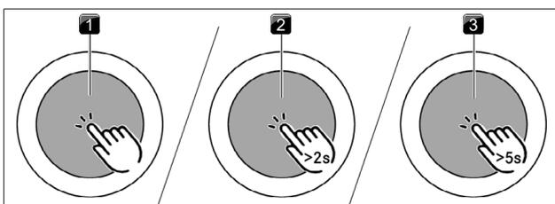
Fig. 5.2 Diagram of the touch commands
