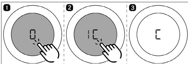
Fig. 5.8 Activating the cooktop extractor cleaning function
