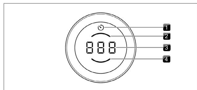
Fig. 3.3 Control knob display elements
