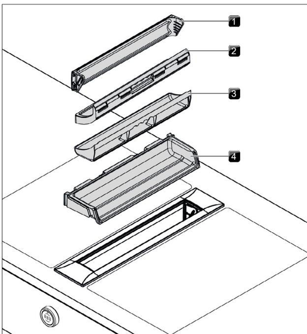
Fig. 3.7 Filter components
