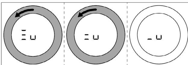
Fig. 5.34 Reducing the active heat retention level
