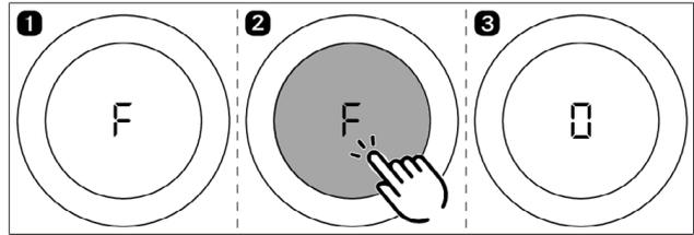
Fig. 5.22 Deactivating the filter service display for a cooking session
