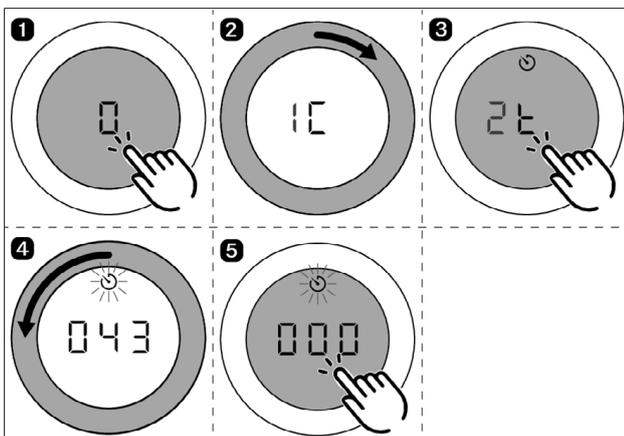
Fig. 5.14 Switching off the short-time timer early
