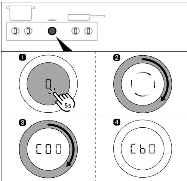
Fig. 6.5 access the configuration menu
