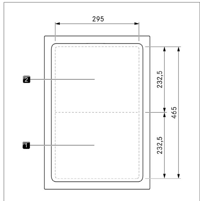
Fig. 3.14 Layout of Tepan stainless steel grill PKT3 and cooking zone dimensions
