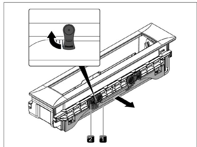
Fig. 7.4 Removing the maintenance tray
