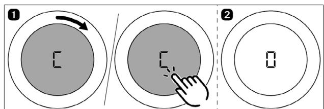
Fig. 5.10 Deactivating the cooktop extractor cleaning function
