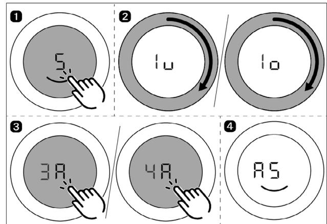
Fig. 5.39 Activating the automatic heat up function
