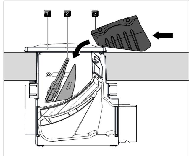
Fig. 7.3 Fitting the cover flap
