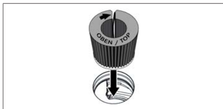
Fig. 7.7 Inserting the activated charcoal filter through the vent opening
