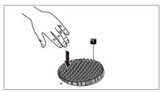
Fig. 7.1 Removing air inlet nozzle PUXA, PUXU
