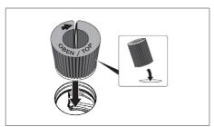
Fig. 7.10 Inserting the activated charcoal filter through the vent opening
