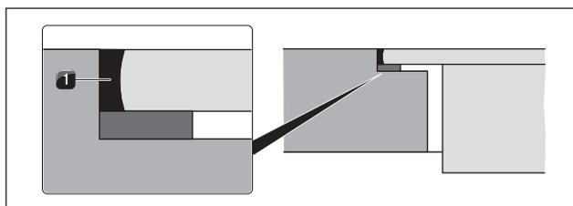
Fig. 5.25 Silicone sealant for flush installation
