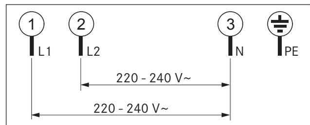
Fig. 5.23 Connection diagram 2-phase
