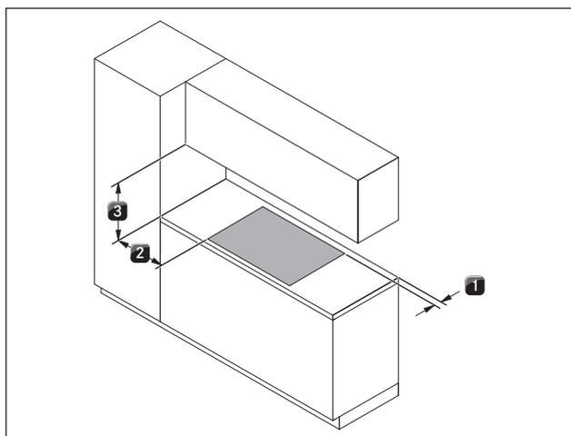
Fig. 5.17 Minimum clearances for installation rotated by 180°
