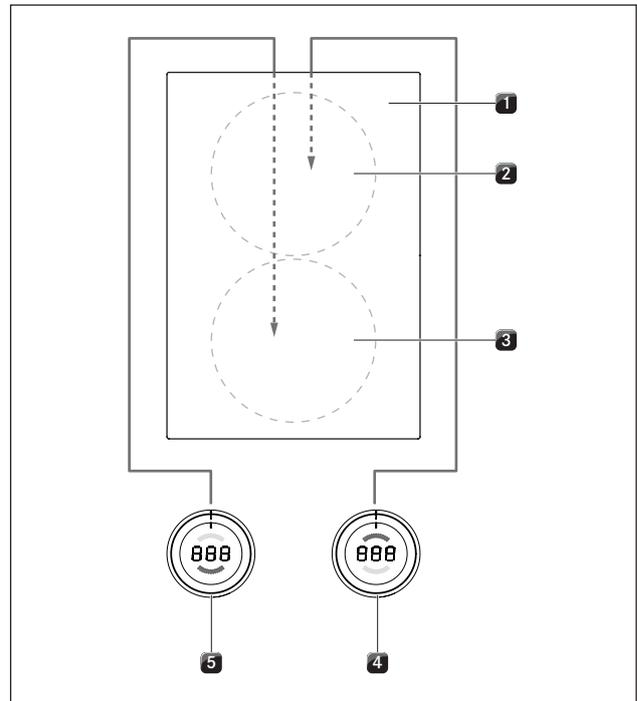
Fig. 5.21 Cooking zone connection in 180° installation
