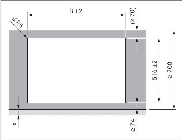
Fig. 5.5 Cut-out dimensions for surface mounting
