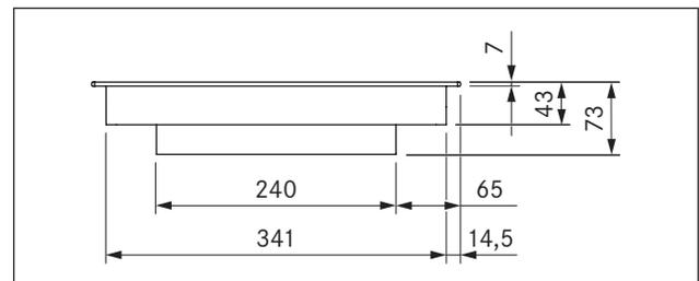
Fig. 3.3 PKCH2 Device dimensions front view
