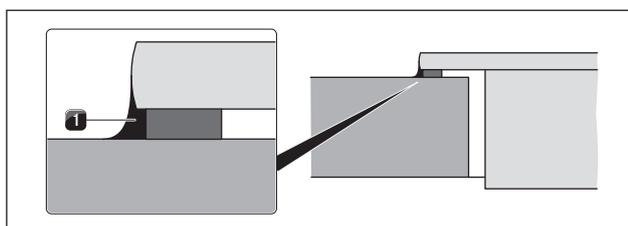
Fig. 5.26 Silicone sealant for surface mounting
