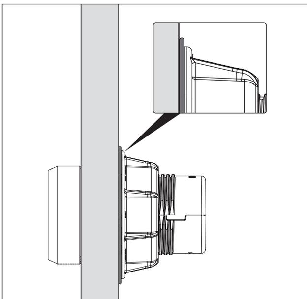
Fig. 5.11 Wave spring once assembly is complete
