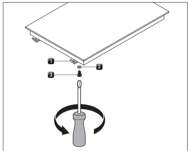
Fig. 5.16 Mounting brackets
