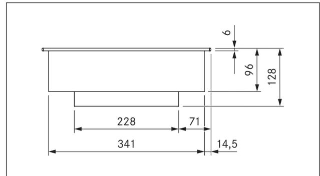
Fig. 3.3 PKIW1 Device dimensions front view
