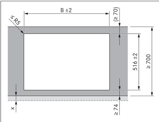
Fig. 5.5 Cut-out dimensions for surface mounting
