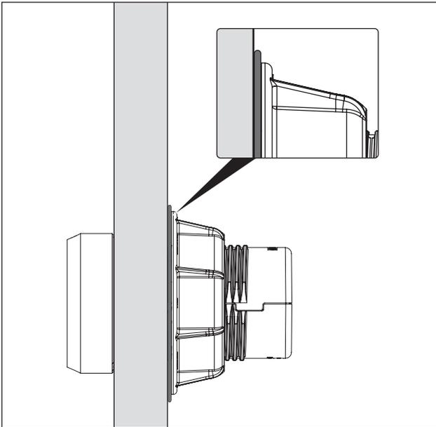
Fig. 5.14 Wave spring once assembly is complete
