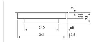
Fig. 3.21 PKCB3 appliance dimensions front view
