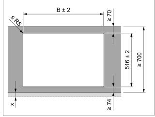
Fig. 4.13 Cut-out dimensions for surface mounting
