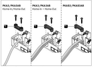
Fig. 4.68 Fitting the strain relief clamp
