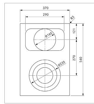
Fig. 3.20 PKCB3 appliance dimensions from above
