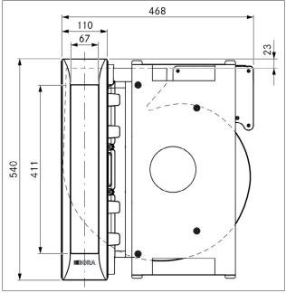
Fig. 3.5 PKAS3/PKAS3AB appliance dimensions from above
