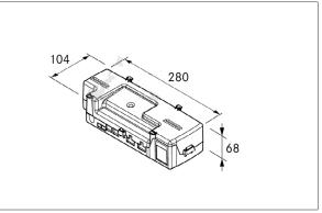
Fig. 3.4 Control unit dimensions
