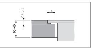
Fig. 4.12 Rebate dimensions for flush installation
