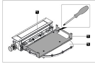
Fig. 4.24 Removing the holding plate
