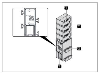
Fig. 4.35 Mounting bracket - left side (surface mounting)
