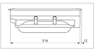
Fig. 3.3 PKA3/PKA3AB appliance dimensions side view
