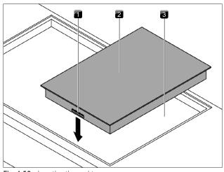
Fig. 4.52 Inserting the cooktop
