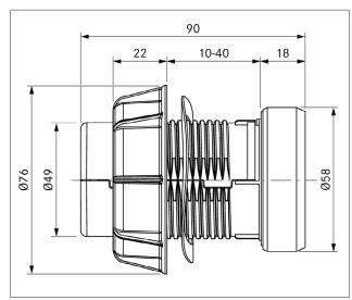
Fig. 3.33 Control knob dimensions
