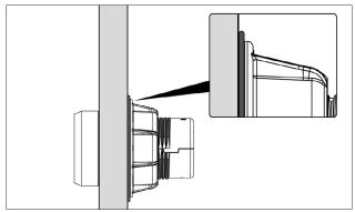
Fig. 4.23 Wave spring when installation is complete
