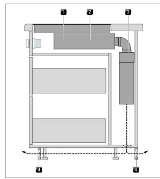
Fig. 4.9 Example of recirculated-air-return-flow planning
