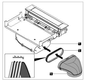
Fig. 4.42 Connecting to the duct system
