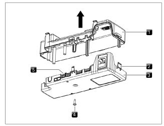
Fig. 4.59 Opening the control unit housing cover
