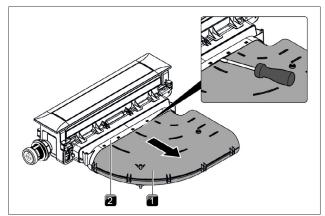
Fig. 4.25 Disassemble the curved duct piece
