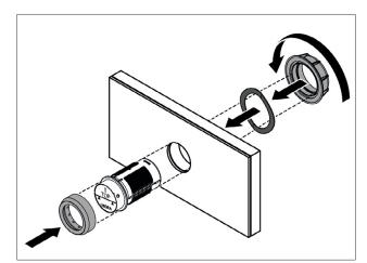
Fig. 4.22 Fitting the control knob
