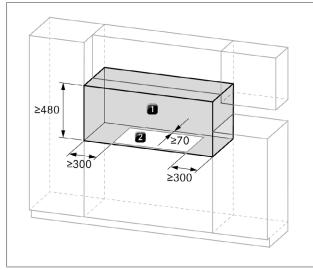
Fig. 4.57 Required clearance
