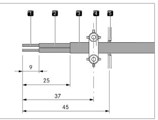
Fig. 4.60 Stripping lengths and installation position of the PKA3/ PKA3AB connection cable
