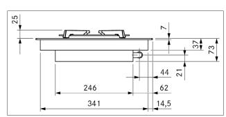
Fig. 3.30 PKG3 appliance dimensions front view
