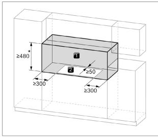
Fig. 4.3 Required clearance
