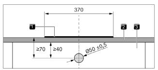
Fig. 4.18 Drilling pattern for wok cooktop with 1 control knob
