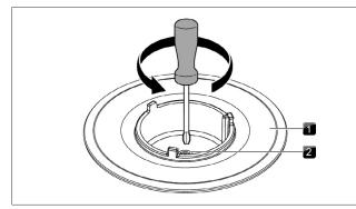
Fig. 4.49 Cooktop burner with gas burner nozzle
