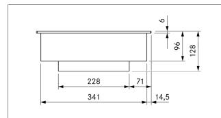
Fig. 3.15 PKIW3 appliance dimensions front view
