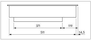
Fig. 3.16 PKIW3 appliance dimensions side view
