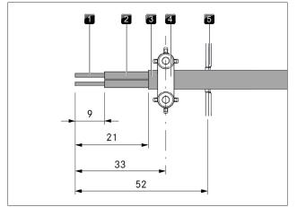
Fig. 4.61 Stripping lengths and installation position of the PKAS3/ PKAS3AB connection cable – Home In
