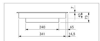
Fig. 3.24 PKCH3 appliance dimensions front view
