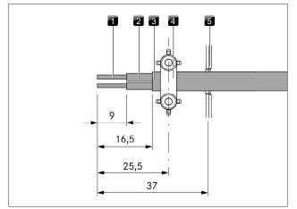
Fig. 4.62 Stripping lengths and installation position of the PKAS3/ PKAS3AB connection cable – Home Out
