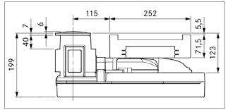
Fig. 3.6 PKAS3/PKAS3AB appliance dimensions front view
