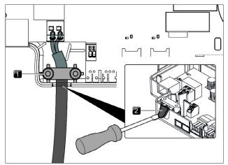
Fig. 4.67 Home Out contacts with strain relief
