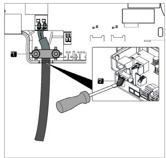
Fig. 4.65 Home Out contacts with strain relief
