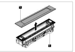
Fig. 4.30 Removing the cover frame
