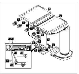
Fig. 4.84 PKA3 connection diagram
