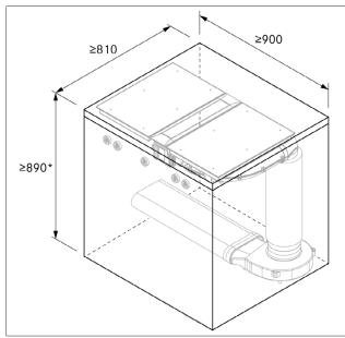
Fig. 4.4 Minimum installation dimensions for standard set-up of PKA3/PKA3AB
