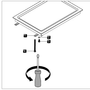
Fig. 4.56 Mounting brackets
