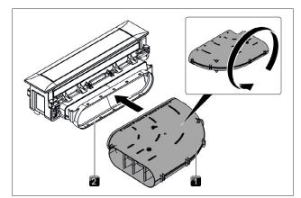
Fig. 4.27 Turning the curved duct piece over
