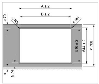
Fig. 4.11 Cut-out dimensions for flush installation
