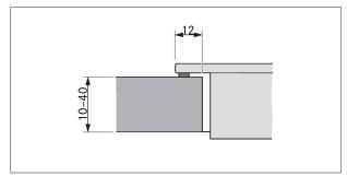
Fig. 4.14 Overlay dimensions for surface mounting
