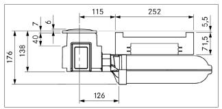
Fig. 3.2 PKA3/PKA3AB appliance dimensions front view
