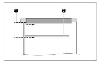
Fig. 4.7 Air supply at front of the unit
