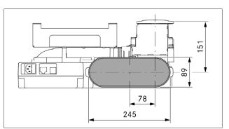
Fig. 4.41 Duct connection dimensions for PKAS3, PKAS3AB
