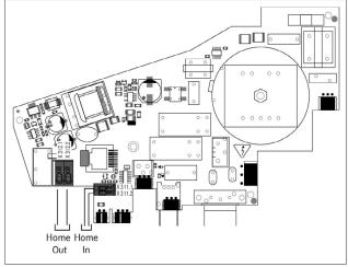
Fig. 4.64 Connection diagram for the external switch contacts
