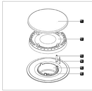
Fig. 4.48 Gas burner structure
