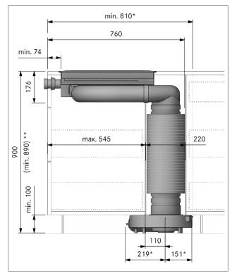
Fig. 4.5 Appliance installation dimensions for standard set-up of PKA3/PKA3AB with round silencer
