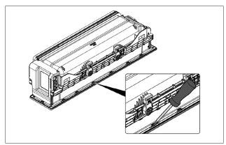
Fig. 4.29 Removing the cover frame
