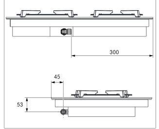
Fig. 4.45 Position of gas connection
