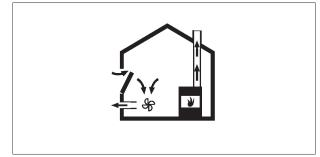
Fig. 4.2 Exhaust air installation - correct
