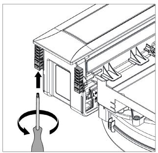
Fig. 4.37 Tightening the mounting clamps
