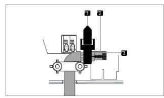
Fig. 4.66 PKAS3 Home-In interface cable tie
