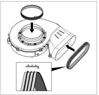
Fig. 4.43 Fitting the seals on the plinth fan
