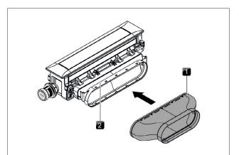
Fig. 4.26 Installing the straight duct piece
