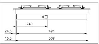
Fig. 3.31 PKG3 appliance dimensions side view
