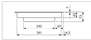
Fig. 3.18 PKC3 appliance dimensions front view
