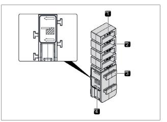
Fig. 4.34 Mounting bracket - right side (flush installation)
