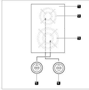
Fig. 4.74 Standard connection of appliances that connect at the front (PKG3)
