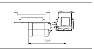
Fig. 4.40 Duct connection dimensions for PKA3/PKA3AB with the straight duct piece
